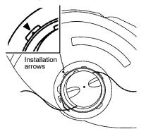
Twist the shield as illustrated until it snaps securely into place. Make sure the shield is assembled to the unit as shown in the illustration below and in the KNOW YOUR TRIMMER section of this manual.
